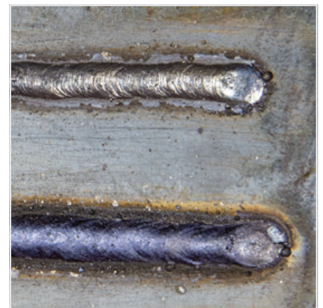
(8) Wait for the weld to cool and carefully chip away the slag to reveal the weld metal below.
