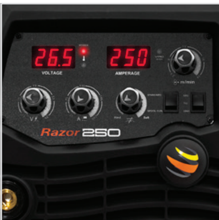
(15) Set welding parameters using the voltage and wire feed controls.
