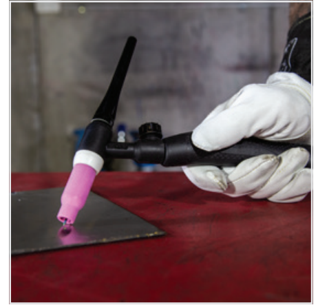
(3) Lay the outside edge of the Gas Cup on the work piece with the Tungsten Electrode 1- 2mm from the work piece.
