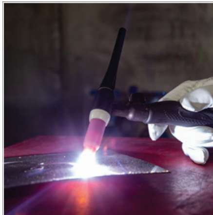
(5) Now rotate the Gas Cup in the reverse direction to lift the Tungsten electrode from the work piece to create the arc.
