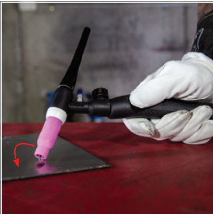
(4) With a small movement rotate the Gas Cup forward so that the Tungsten Electrode touches the work piece.
