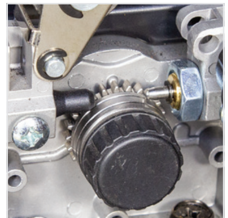
(9) Install a U groove drive roller of the correct size for the diameter wire being used.
